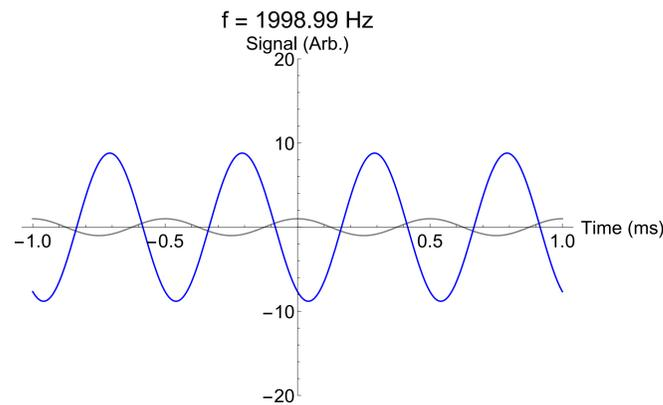
Figure 1: Signal vs. Time (ms). The gray signal represents the reference from the function generator, and the blue signal represents the signal from the microphone.
