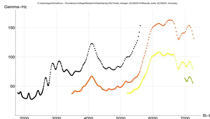
Figure 5: Resonance Peak Width (Hz) vs Frequency (Hz) for Nitrogen
