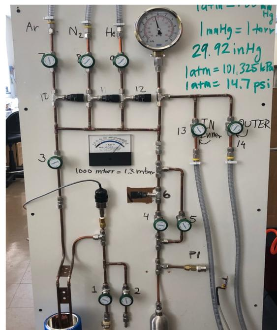
Figure 3: Gas-handling apparatus.
