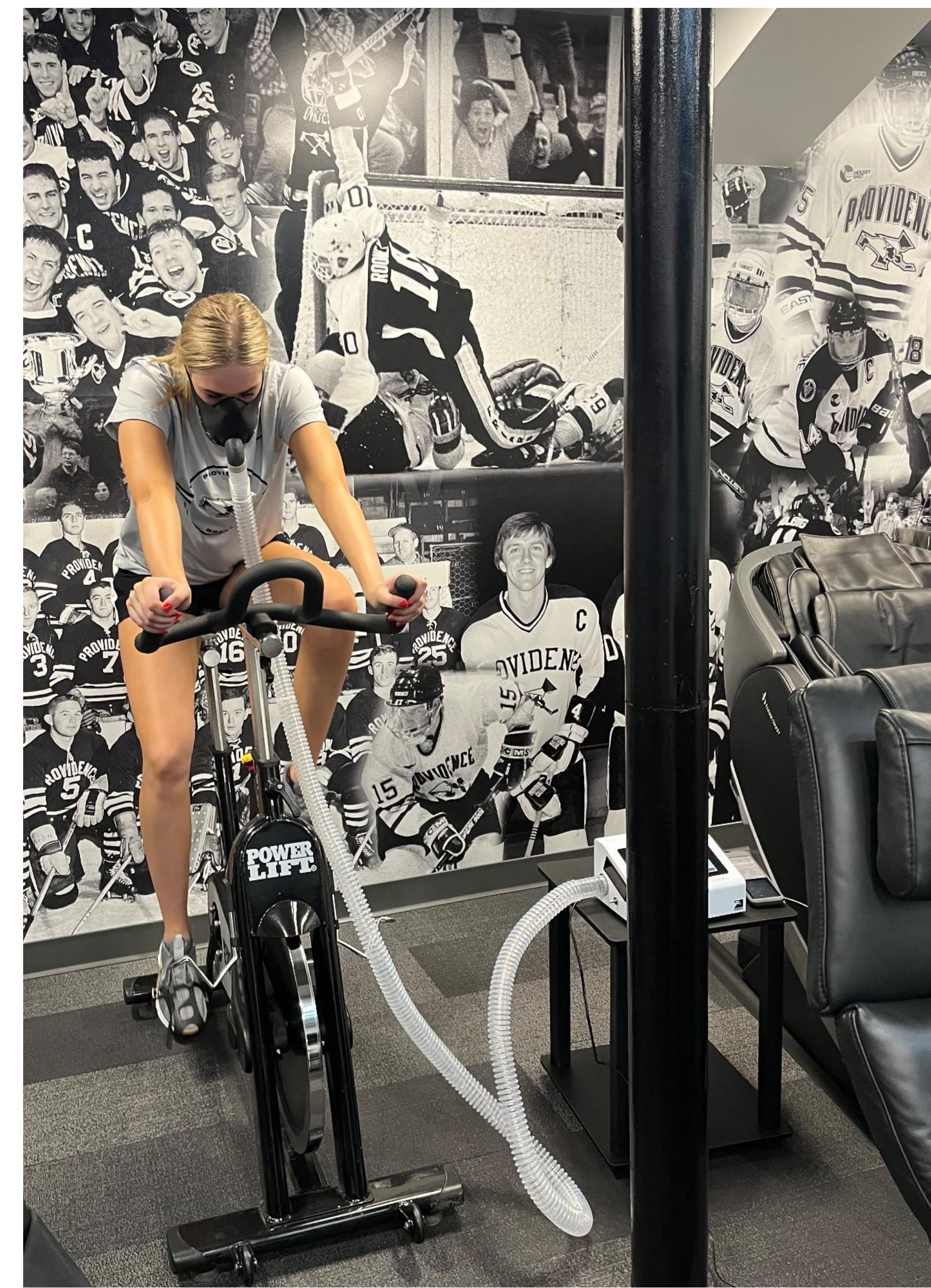
The Apollo system measures oxygen consumption as a way of calculating energetic expenditure.
