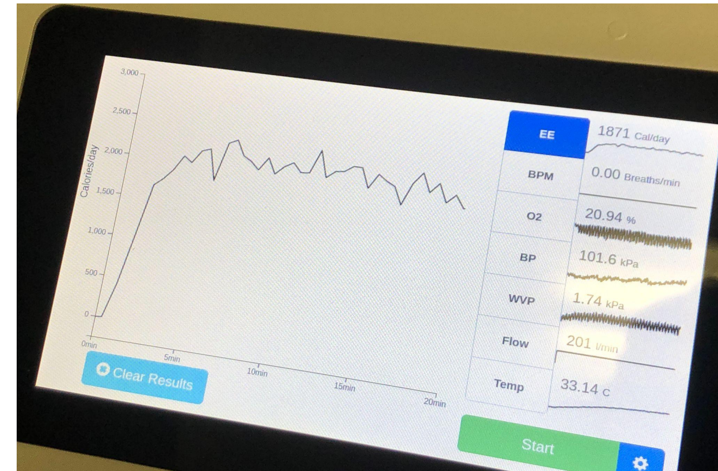
The Apollo system measures oxygen consumption as a way of calculating energetic expenditure.
